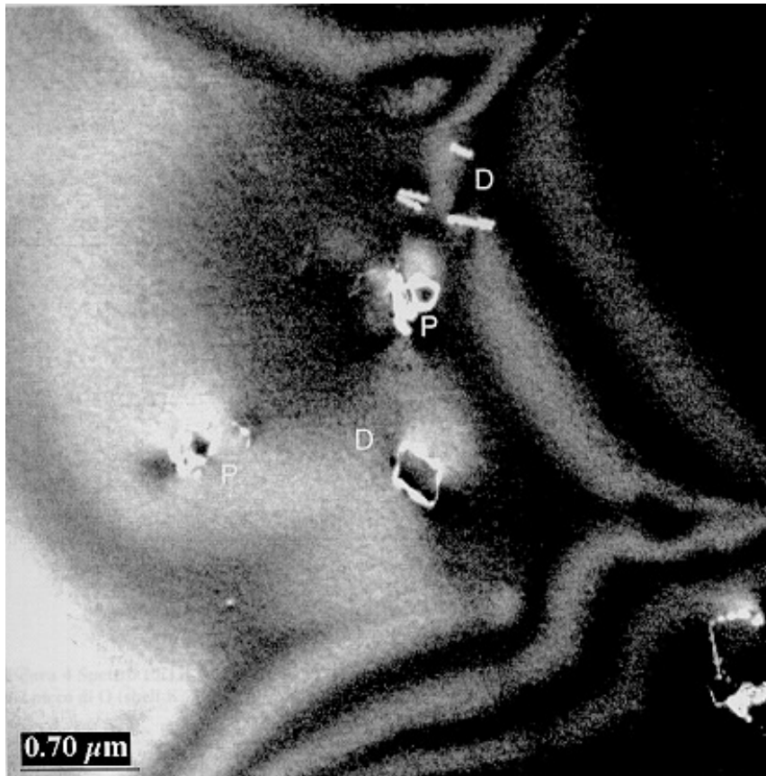
Figure 3. TEM micrograph of precipitates (P) and planar defects (D), consisting of dislocations decorated by small precipitates.
